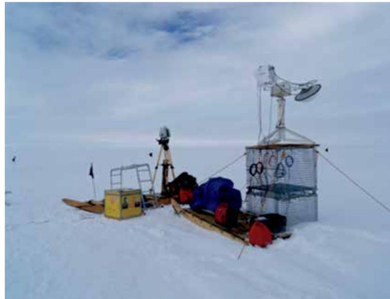
Figure 1. On-site measurements of the scatterometer and lidar from the snow-covered sea ice at Cambridge Bay, Nunavut on May, 2014.
