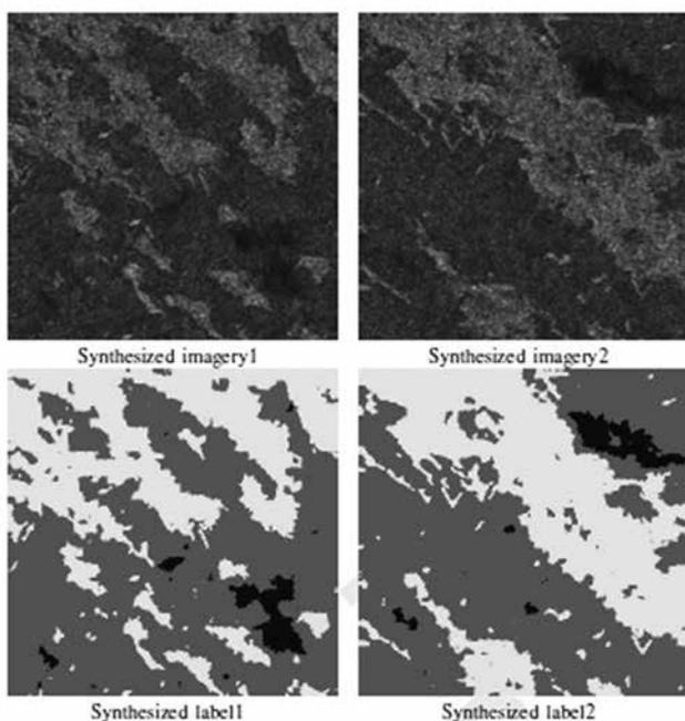
Figure 5. Two examples of synthesized SAR scenes with ice, water, and oil and accompanying scene with labels.
