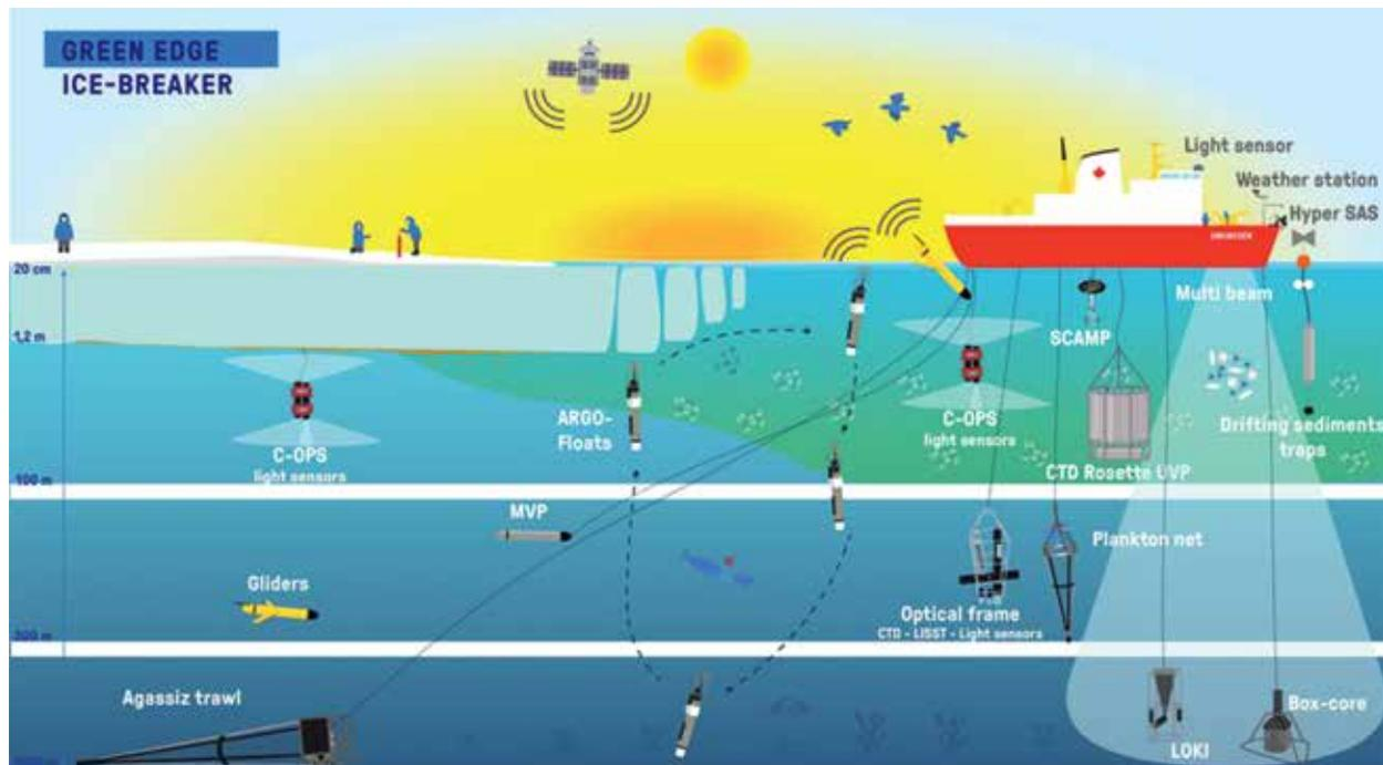
Figure 4. Visual summary of the equipment used during the GreenEdge oceanographic cruise (credit: Julie Sansoulet).
