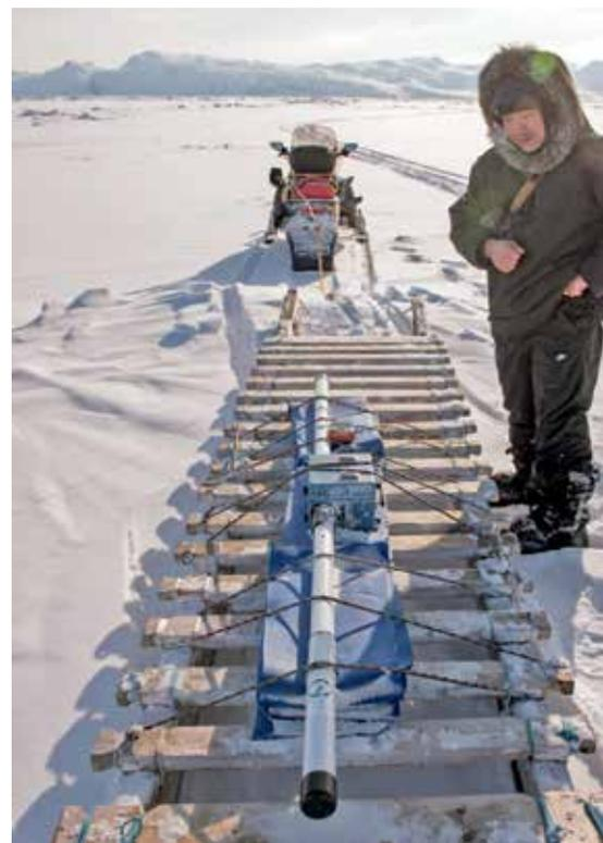
*Figure 2. SmartICE local research coordinator Andrew Arreak using SmartQAMUTIK to measure sea-ice thickness on Eclipse Sound near Pond Inlet, Nunavut (photo: SmartICE 2016).*
