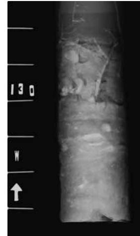
Figure 8. X-ray of trigger-weight core 2016804014 showing bamboo coral fragments immediately above glacial-age diamict, Disko Fan site, ~913 m water depth.
