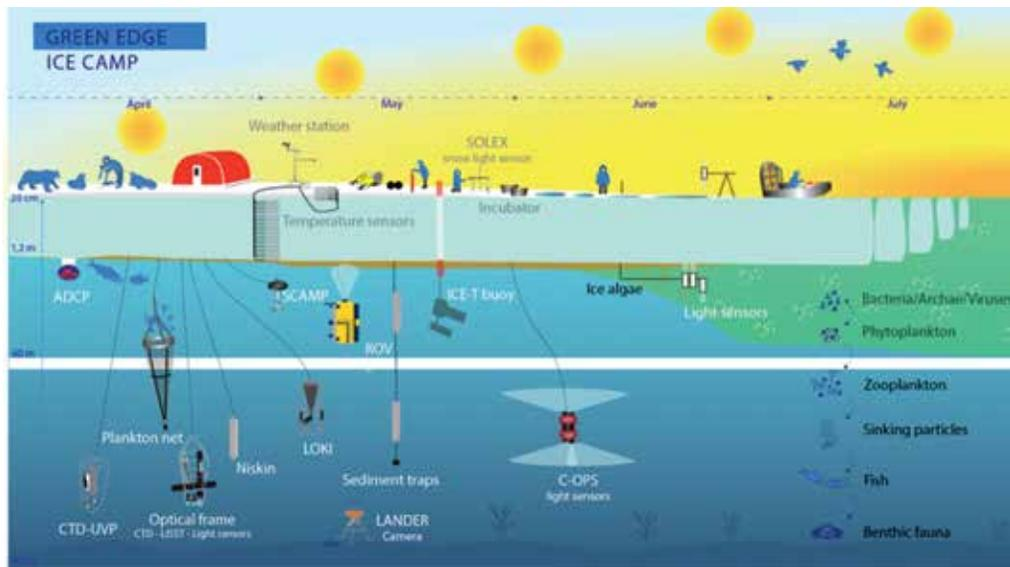
Figure 2. Visual summary of the instruments used during GreenEdge ice camp operations in 2016 (credit: Julie Sansoulet).
