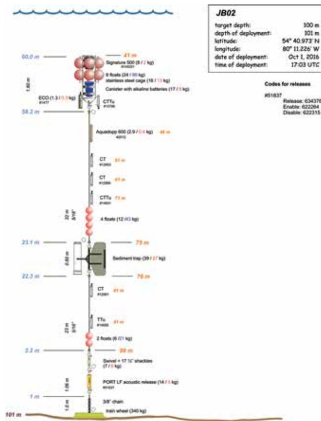
Figure 2. Mooring diagram for the mooring installed at the mouth of James Bay October 1, 2016, in partnership with the NSERC BaySys CRD project (D. Barber, Lead).
