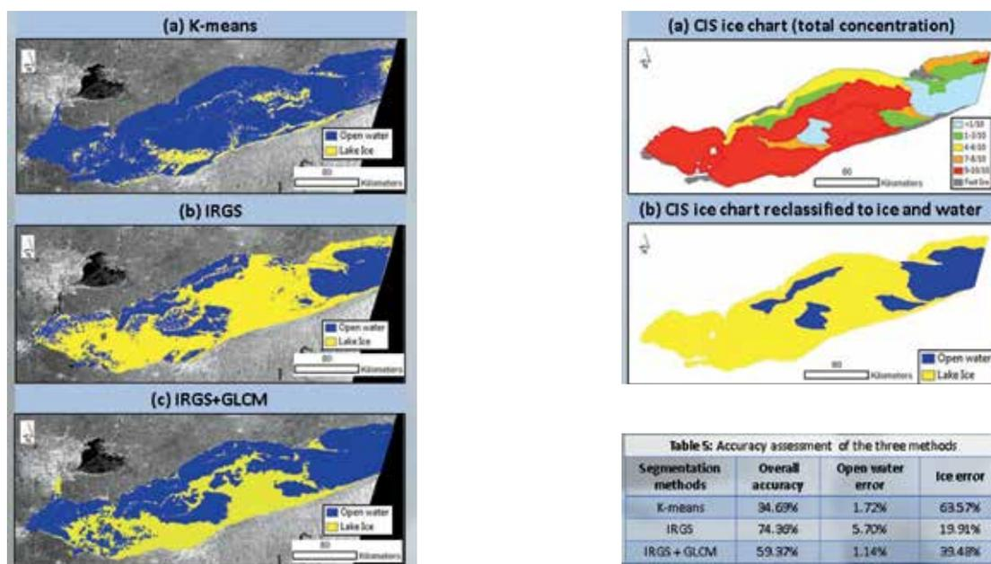
Figure 6. A comparison of classification tests for lake ice SAR scene. K-means, IRGS, and IRGS + texture features are compared with the later showing the best performance.
