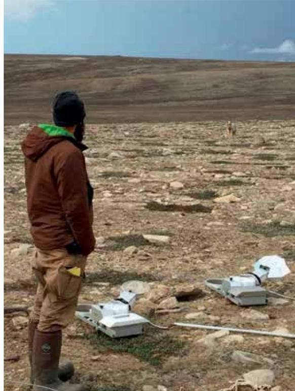
Figure 1. Automated chamber systems measuring net carbon dioxide fluxes from polar semi-desert communities at the CBAWO. Even the wildlife like to observe research. Photo by Robert Mactavish.
