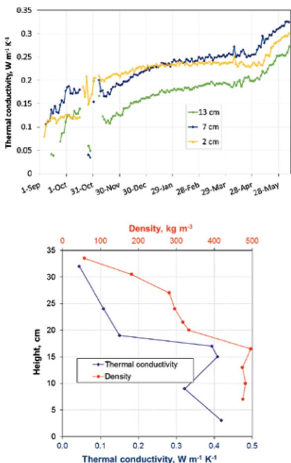
Figure 5. Measurement of snow physical properties at Ward Hunt Island. Top: continuous thermal conductivity measurements at three heights above ground, showing high values even at the very base of the snowpack. Bottom: vertical profile of snow density and thermal conductivity on thin rocky soil at a nearby spot (Source: Florent Domine, CEN/ArcticNet).
