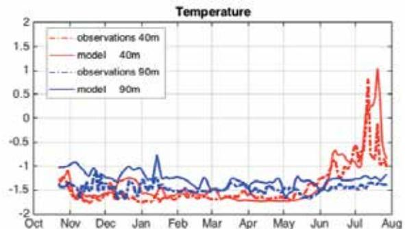
Figure 4. Modeled output (plain line) and observed (dash line) temperatures at 40 m (red) and 90 m (blue) at CA04 from October 2007 to August 2008.
