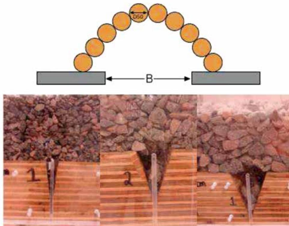
Figure 11. Soil particle bridging sketch and laboratory testing photos. Note the definition of bridging ratio is the width of gap ( $B$ ).
