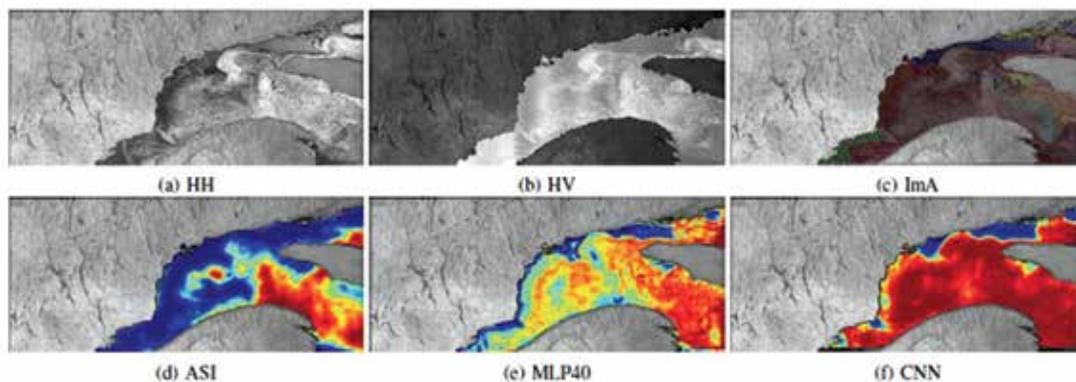
Figure 2. Similar to Figure 1, but showing a different SAR scene. The results again demonstrate the superiority of the CNN method to produce more detailed ice concentration maps.
