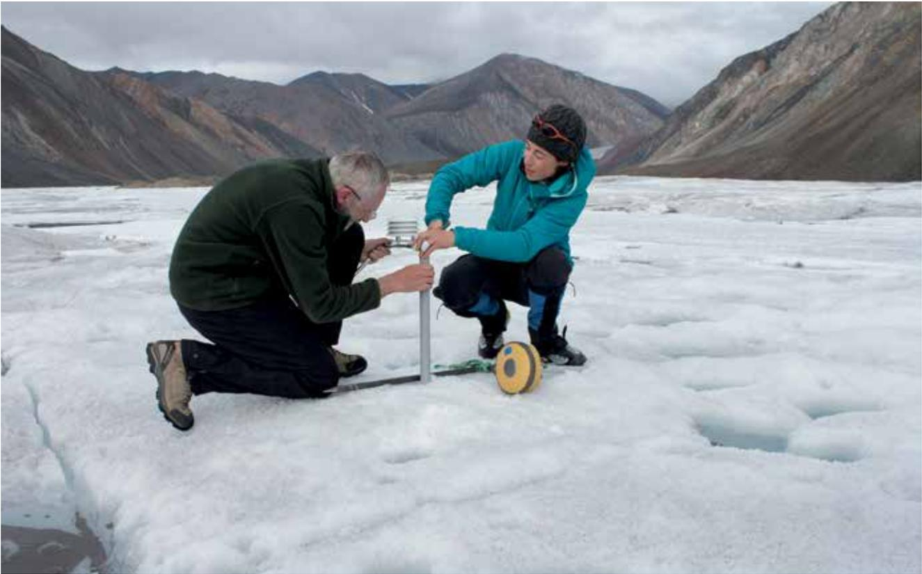
Figure 3. ArcticNet student Jill Rajewicz and Adjunct Professor Greg Crocker install a temperature sensor on an ablation stake on the Milne Glacier (Photo credit: Mike Taekema, ArcticNet).
