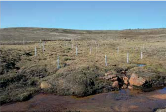
Figure 14. Field site with installed piezometers that provide measurements of the water level below the soil surface.
