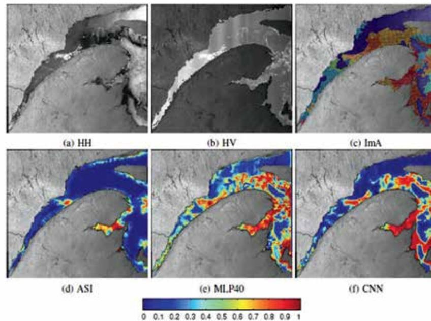
Figure 1. The ice concentration estimation result by CNN compared to ASI and MLP40 ice concentration for SAR scene. (a) and (b) represent the HH and HV pols, (c) is the corresponding image analysis chart, (d) represents the results using the known ASI algorithm, (e) represents results using a neural network MLP40, and (f) is the result using our designed CNN. Our CNN method provides a more realistic and accurate interpretation of the ice concentration.
