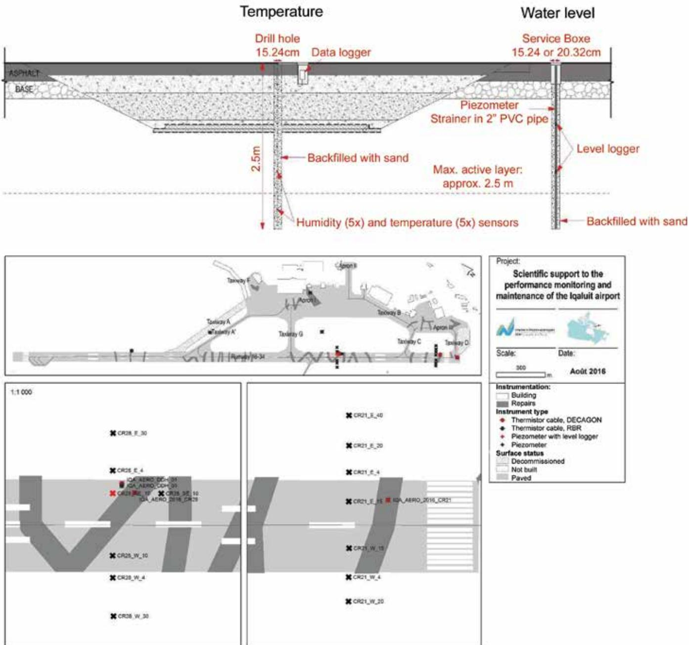
Figure 10. Thermistor cables installed in repaired cracks across the runway in Iqaluit.
