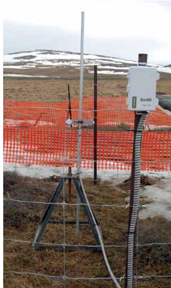
Figure 8. Instrumentation of plots using spectral reflectance probes (SRS, Decagon, Pullman, WA, USA) which allow continuous estimation of the standardized difference vegetation index (NDVI) and the photochemical reflectance index (PRI).
