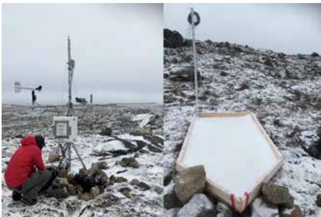
Figure 12. Apex River meteorology station.
