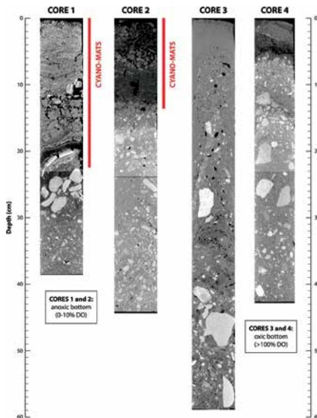
Figure 9. CT-scans of the four sediment cores from Ward Hunt Lake (Photo credit: Frédéric Bouchard, CEN/ArcticNet).
