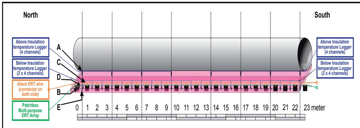
Figure 9. Scheme of the Abem Terrameter LS system used in the electrical resistivity tomography (ERT) surveys.
