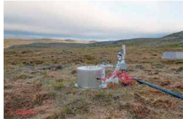
Figure 12. Automated chambers to detect and measure permafrost soil respiration.
