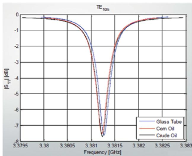
Figure 4. TE105 permittivity measurements of corn oil, crude oil, and a glass tube with cavity over coupling for all three cases using a resonant perturbation method (Chen et al. 2004). Data and figure provided by Thomas Neusitzer (University of Manitoba).
