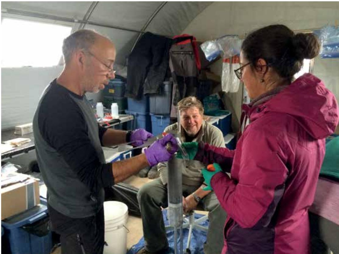
Figure 5. Vincent St. Louis, Charley Talbot (ECCC) and M.Sc. student Maria Cavaco sectioning a sediment core from 263 meters depth in Lake Hazen for biogeochemical and microbial parameters (Credit: J. Serbu).
