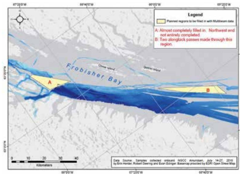
Figure 2. Map showing areas surveyed using multibeam sonar aboard CCGS Amundsen, July 14-27, 2016.
