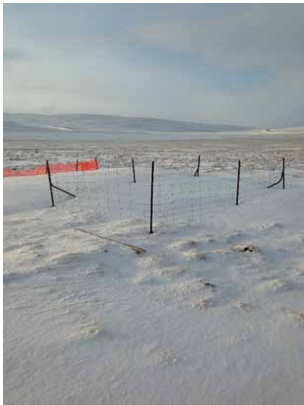
Figure 9. An enclosure located downwind from one out of nine snow fences erected at Deception Bay, Nunavik, in July 2015 to simulate the indirect effects of the development of the shrub layer on snow interception and shading of ground layer plants (shading tarp not installed on this picture). A second enclosure without a snow fence is also present at each experimental site (not visible on the picture).
