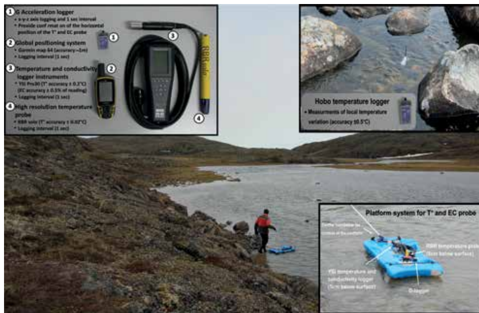
Figure 6. Temperature and conductivity profiling. An instrumented floating platform was trawled along channel margins to detect local anomalies in temperature and electrical conductivity (photo by G. Chiasson-Poirier).
