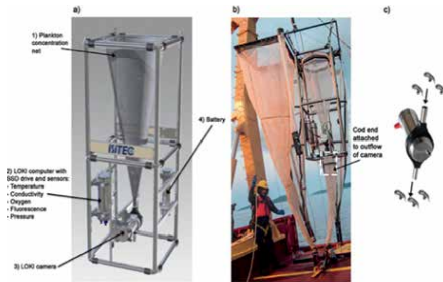
Figure 2. The LOKI in situ zooplankton imager (left) and its deployment from the Amundsen as a component of the zooplankton multiple-net vertical sampler (right).
