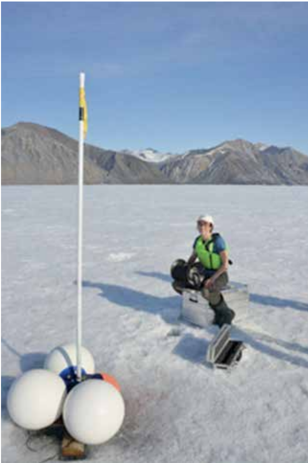
Figure 2. MSc student Jill Rajewicz making a CTD profile of the epishelf lake in July 2015. This oceanographic mooring has been monitoring Milne Fiord since May 2011 is on the left. (Photo by Adam Garbo).
