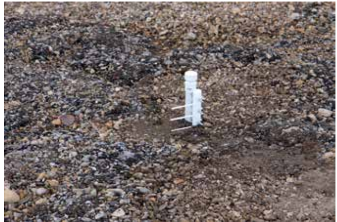
Figure 1. Post holding the three heated needle probes at heights of 2, 8 and 14 cm and the three thermistors at heights of 0, 6 and 12 cm. Cables linking the instruments to the data logger have been buried to protect them from wildlife. (Photo by Denis Sarrazin).
