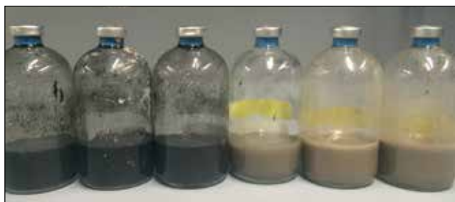
Figure 8. Diesel-amended microcosms of Cambridge Bay sediments incubated under cold anoxic conditions turned black after eight weeks (left), compared to no-diesel unamended controls (right). The other six diesel amended sediments from other locations were similar in appearance to the controls (not shown).
