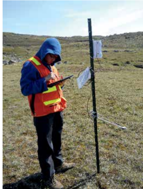
Figure 10. Instrumentation for deriving the fraction of photosynthetically active radiation (FAPAR) - data logger (white box), PAR sensor looking down. These data are compared to another PAR sensor looking upward to collect total incident PAR. (photo by R. Edwards).
