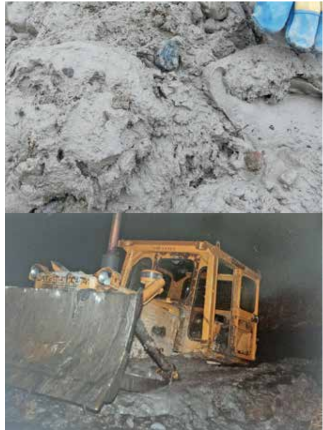
Figure 7. (top) Thixotropic sandy silt or silty sand, known locally as aimayumaima, is unsatisfactory as foundation material – surficial sediment mapping is important to determine the origin and distribution of this unit. (bottom) Loading thixotropic sediment with equipment or a building can result in a loss of bearing capacity.
