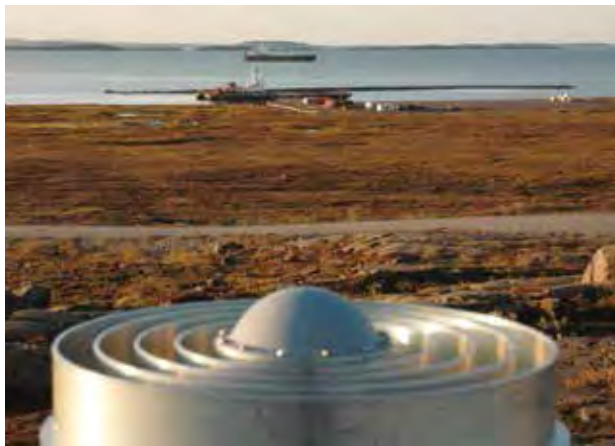
FIGURE 19. Port facility (wharf and offshore breakwater) at Kugluktuk, NU, 2009 with tug and barge alongside, and pipeline (narrow white line) running up the slope to the fuel tanks (out of view to right). Sea-lift freighter out of Montréal in background. Global Navigation Satellite System (GNSS) antenna in foreground used to measure vertical land motion (Forbes et al. 2004; Couture et al. 2014; James et al. 2014).
