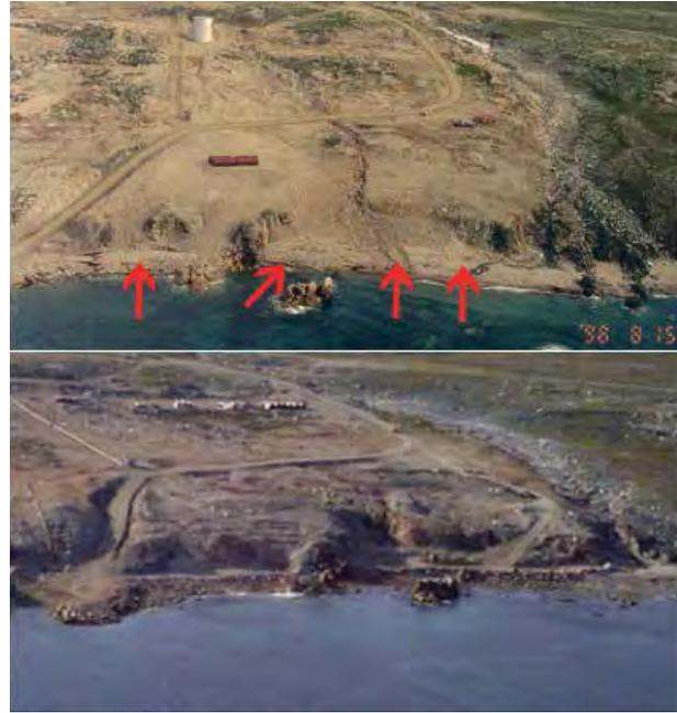
**Figure 3.** Beach area in Saglek Anchorage before (top, 1996) and after (bottom, 1999) contaminated sediment excavation and removal. The volume of sediment removed was 16,240 m<sup>3</sup> (arrows indicate where sediment was removed), enough to cover a Canadian football field to a depth of around 4 m). Runoff and sediment erosion carried PCBs offshore into the bay.
